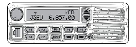
The Vertex Standard **VX-1400** is a low-cost, rugged, small size, integrated HF communications transceiver designed for the worldwide Land Mobile, Government, and Marine markets. The **VX-1400** conforms with MIL-810 C, D, E, & F. The front panel is water resistance to IP54 specifications when in remote control operation using the optional **RMK-1400** Remote Mounting Kit with the **MH-77**ABJ/BBJ Water Resistance Hand Microphone.
