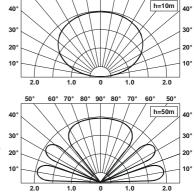
dipole at a height of 10 meters could, ionospheric propagation conditions permitting, be expected to provide outstanding performance over the same 3000 km distance.
