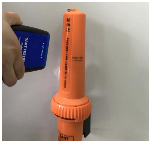
Figure 5-6. SART measurement process
