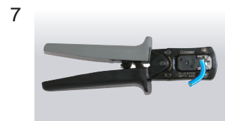
Using special crimping tool MPT5-8AS (PANDUIT CORP.), crimp the modular plug. Finally check the plug visually.
