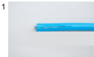
Expose inner vinyl sheath.
